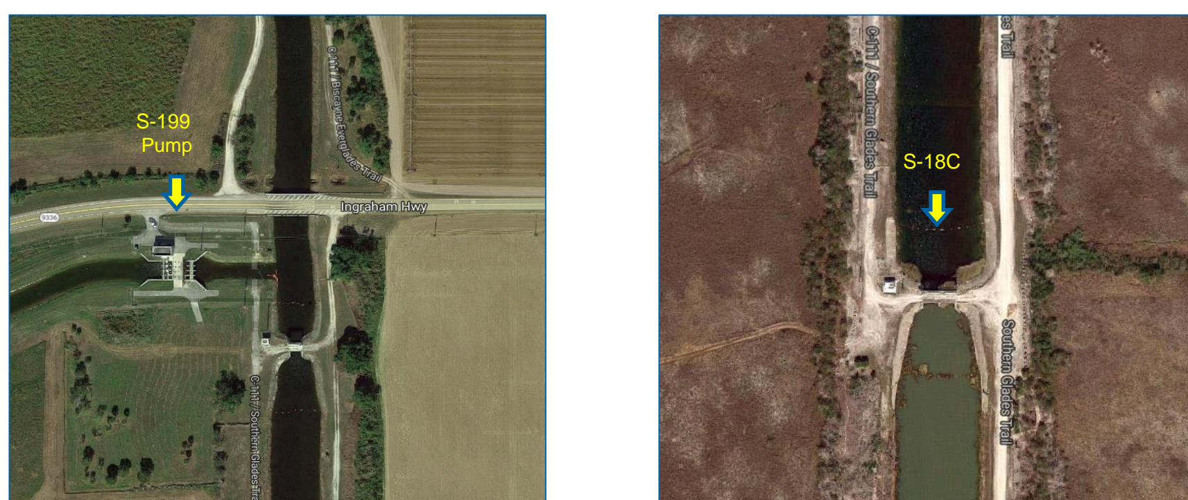
Figure 2. Left photo, Pump S-199, directs C-111 flows into Taylor Slough via secondary canal. S-199 has been operational since February 2012. Right photo, Spillway S18C with controls C-111 flows south to the EP and S-197 leading into Manatee Bay
